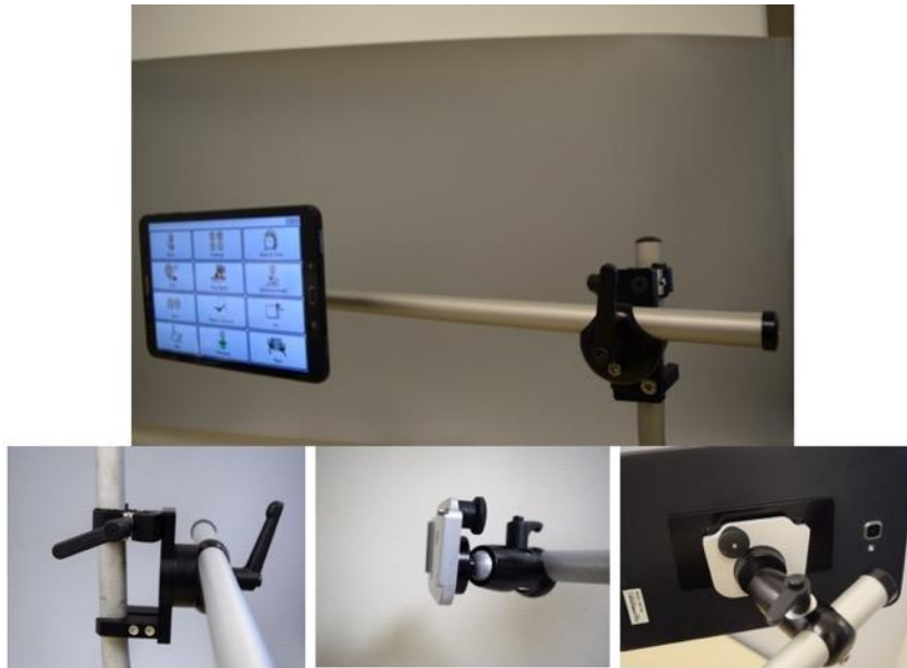
Figure 27 Tablet Mounting arm and quick release bracket at the end of the adjustable swivel head
