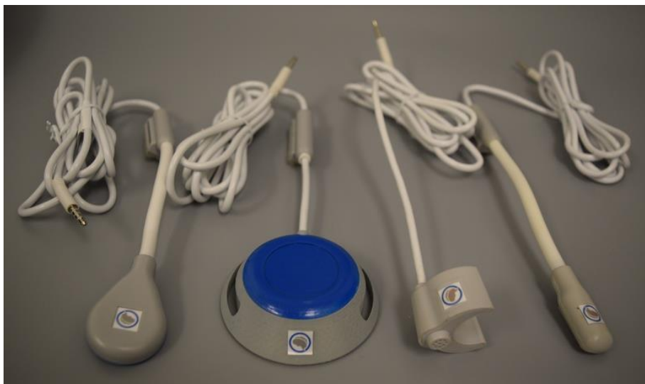
Figure 7: (Left to right) J-Touch, Bed-Touch, Vent-Mic, J-Mic.
