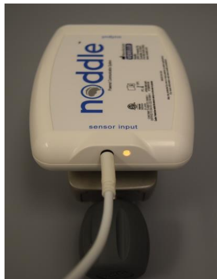
Figure 19: The noddle indicating that the response has been cancelled after being activated 4 or more times by intentional gestures.
