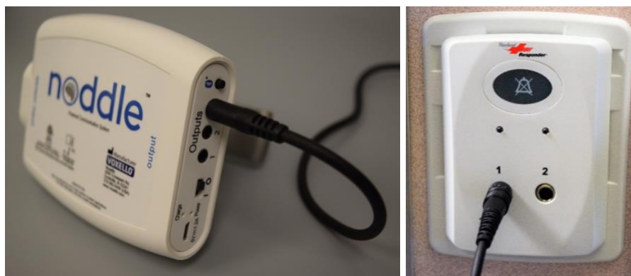
Figure 9. Left: Nurse call cable plugged into the back of the noddle; Right: Nurse call cable plugged into headwall.
