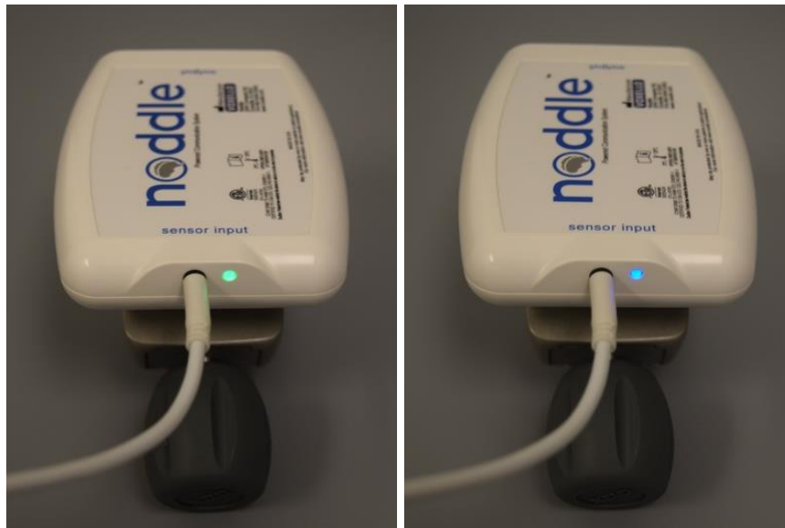
Figure 18: The noddle responds to an intentional gesture by flashing green (left) and then blue (right) for each activation.
