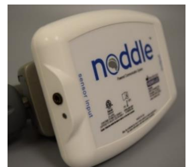
Figure 2: Front side of noddle with input jack and selection indicator light
