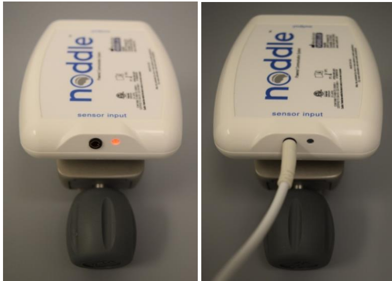
Figure 17: noddle waiting for a sensor to be plugged in (left), and with sensor plugged in (right)
