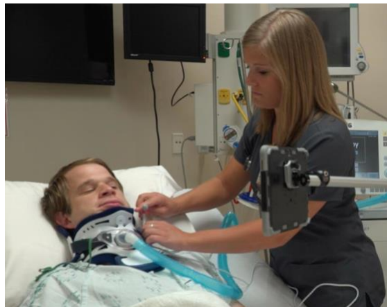
Figure 6: Nurse attaching J-Mic sensor on patient-side mounting site of the sensor
