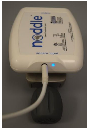
Figure 14: Selection indicator light flashes blue to indicate that the noddle is now in Bluetooth® pairing mode
