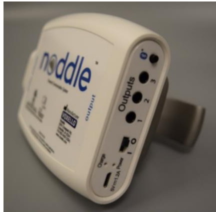
Figure 3: Rear side of noddle with (left to right) power jack, charging indicator light, power on/off indicator light, power switch, input jacks 1-3 and Bluetooth® pairing button.
