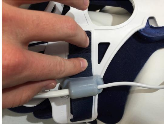
The noddle-mic™ can also be used with an elastic head band. The head band can be pulled through the slot in the noddle-mic™ sensor and adjusted to allow positioning of the sensor so that the patient's tongue clicks activate the noddle™.
