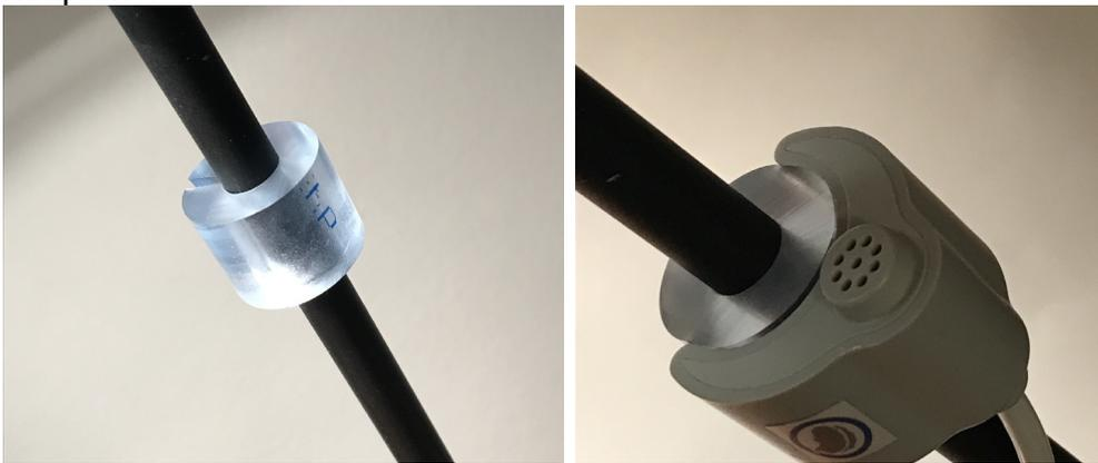
12. Ensure that the microphone is properly positioned so that the patient can easily activate the noddle™ with a tongue click.
