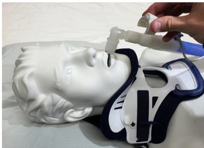
10. The noddle-mic™ should easily snap onto the vent line.
