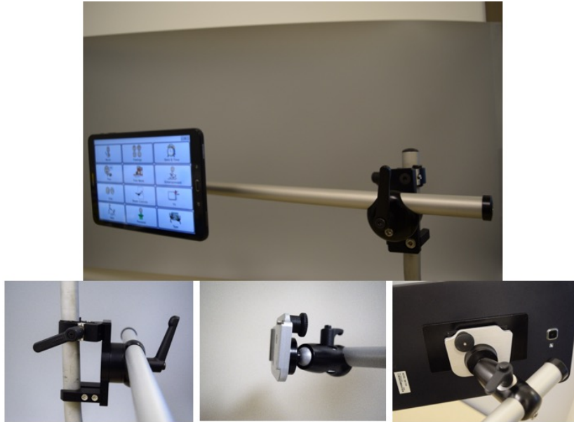
Figure 28: Tablet Mounting arm and quick release bracket at the end of the adjustable swivel head
