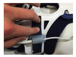
The noddle-mic<sup>TM</sup> can also be used with an elastic head band. The head band can be pulled through the slot in the noddle-mic<sup>TM</sup> sensor and adjusted to allow positioning of the sensor so that the patient's tongue clicks activate the noddle<sup>TM</sup>.
