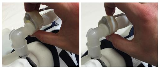
11. The noddle-mic<sup>™</sup> can also be clipped to the vent-line support arm with the supplied adapter.
