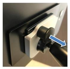
To adjust the angle of the tablet, loosen the lever behind the tablet. Tighten the lever to lock the tablet into position.
