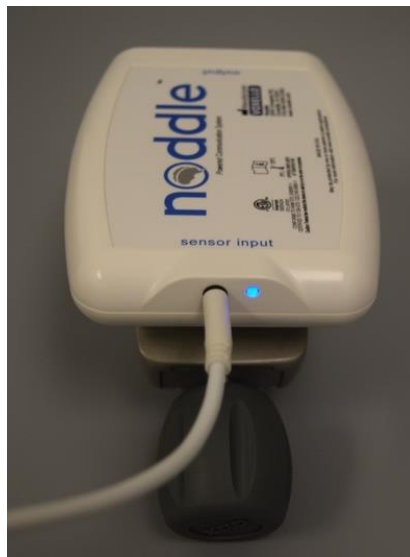
Figure 11: Selection indicator light flashes blue to indicate that the noddle™ is now in Bluetooth® pairing mode
