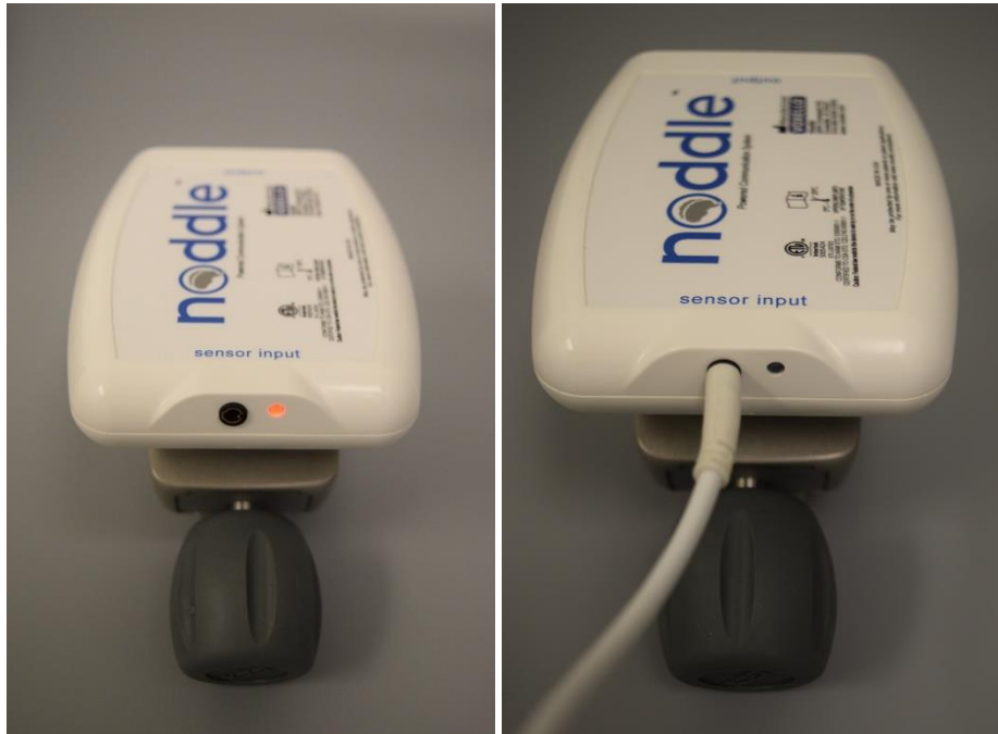
Figure 14: noddle™ waiting for a sensor to be plugged in (left), and with sensor plugged in (right)
