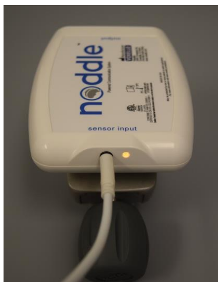
Figure 16: The noddle™ indicating that the response has been cancelled after being activated 4 or more times by intentional gestures.
