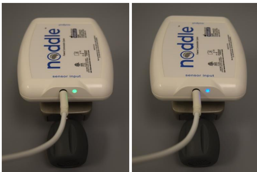
Figure 15: The noddle™ responds to an intentional gesture by flashing green (left) and then blue (right) for each activation.
