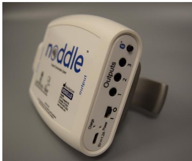
Figure 3: Rear side of noddle™ with (left to right) power jack, charging indicator light, power on/off indicator light, power switch, input jacks 1-3 and Bluetooth® pairing button.
