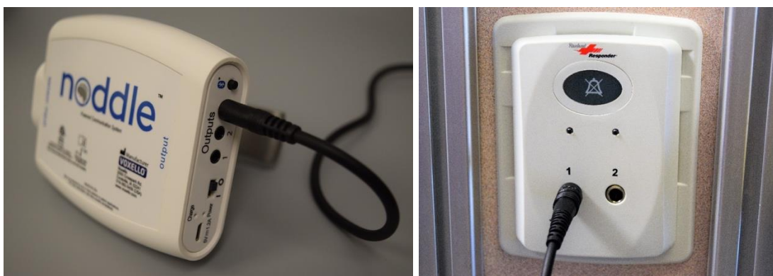
Figure 9. Left: Nurse call cable plugged into the back of the noddle™; Right: Nurse call cable plugged into headwall.
